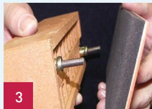
4. Place the rubber washer over the threaded bar. Repeat on the other side.
